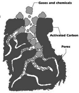
Activated Carbon adsorbs gases and chemicals Applied Ozone Systems Corona Discharge Ozone Generators Ozonators <a href="http://www.appliedozone.com/ozone\_generators\_ozonators.html">http://www.appliedozone.com/ozone\_generators\_ozonators.html</a>
