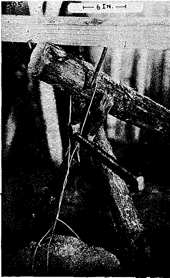
FIG. 331. LOG DOGGED ON ITS TRESTLE TO BE SAWN INTO BOARDS. The squared log already line-marked, to be sawn horizontally into four boards, indicated by parallel lines dimly seen is stapled (doggd) fast upon the top log of one of its trestles.
