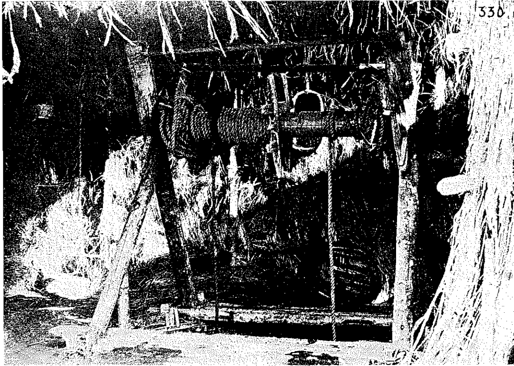
FIG. 2. COAL MINE'S WINDLASS. There are two units of rope in use upon the cylinder of the windlass. When the one is wound, the other is unwound, with the effect that by turning the cranks one rope winds to pull up a load, while the other unwinds to let down an empty basket into the shaft of the mine.
