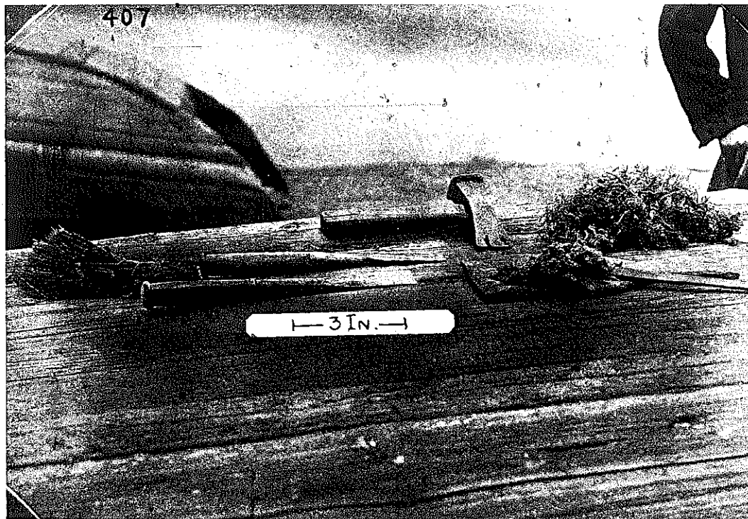
FIG. 504. CHINESE SHIPBUILDER'S CAULKING TOOLS.
