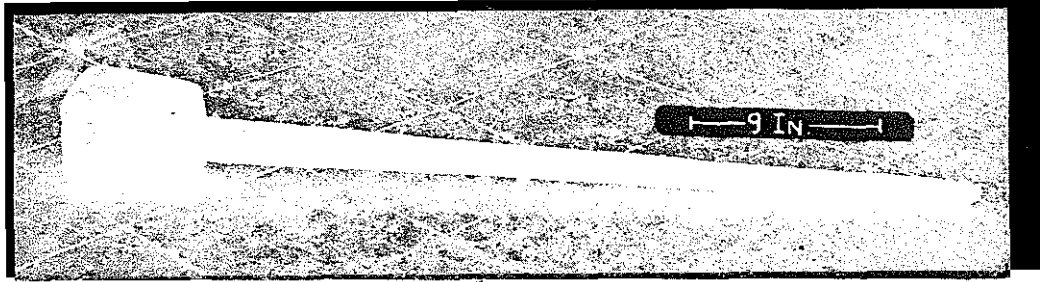
FIG. 432. WOODEN RAMMER USED IN MAKING CHINESE COMPOSITION PAVEMENTS.
