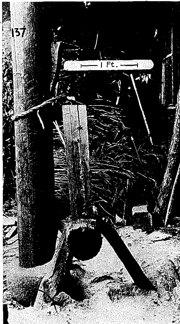
FIG. 532. COOPER'S CLAMP FOR SAWING OUT TUB STAVES.
