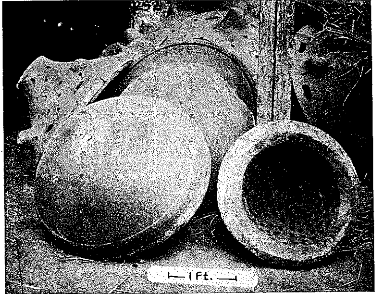
FIG. 44. MOLDS FOR CASTING IRON COOKING BOWLS.
