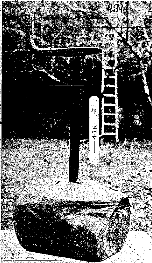
FIG. 530. PEWTERER'S STAKE WITH BLUNT HORNS FOR HAMMERING HOLLOW PEWTER VESSELS INTO FINAL SHAPE. This wrought iron pewterer's stake together with the wooden block into which it has been driven and tightened with molten pewter, is 21½ inches high.
