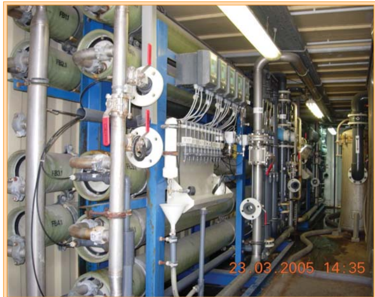
One of the four containerized BWRO trains, Dshanim Factory, Israel.
