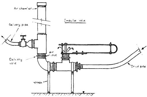
Fig.58 Details of ITDG hydraulic ram
