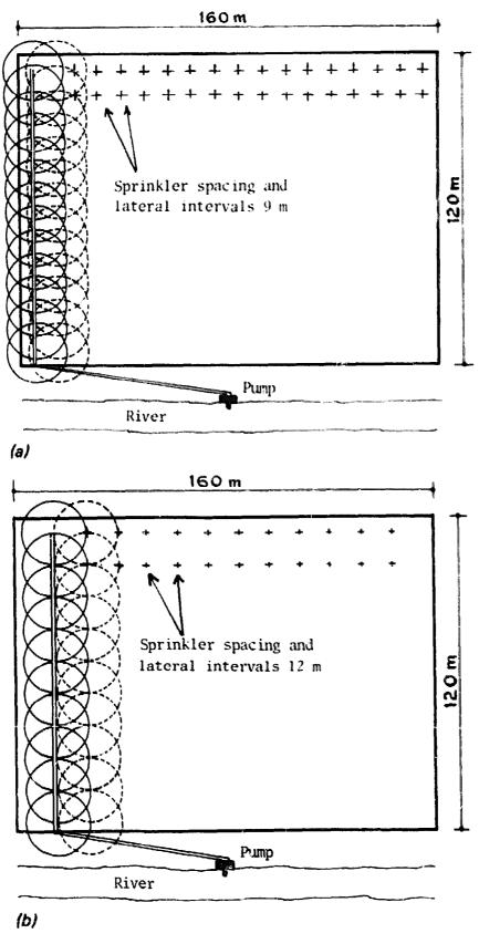
Fig. 22 Possible arrangements for a small sprinkler irrigation system
