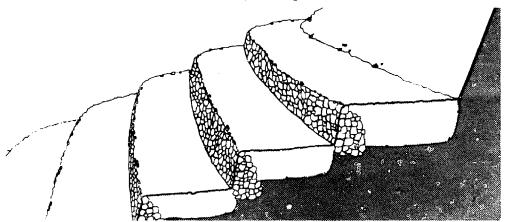
Fig.9 Run-off interception with terraces made of stones
