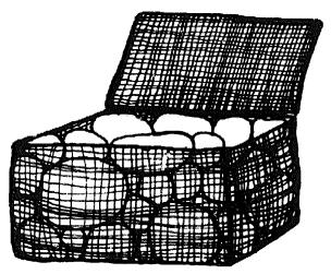
Fig.33 Gabion filled with stone, lid open
