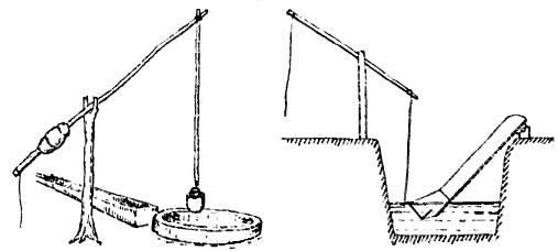
Fig.41 The beam and bucket
