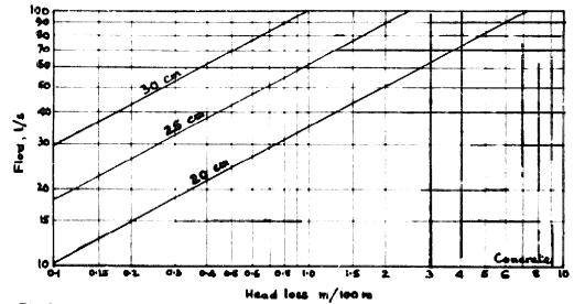
Fig.36 Concrete pipe design chart for various pipe sizes measured by internal diameter
