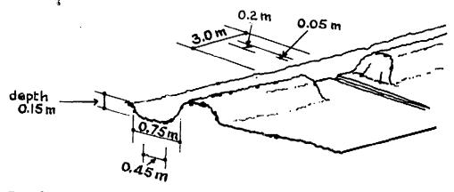
Fig.13 Details of seepage furrows and spillway
