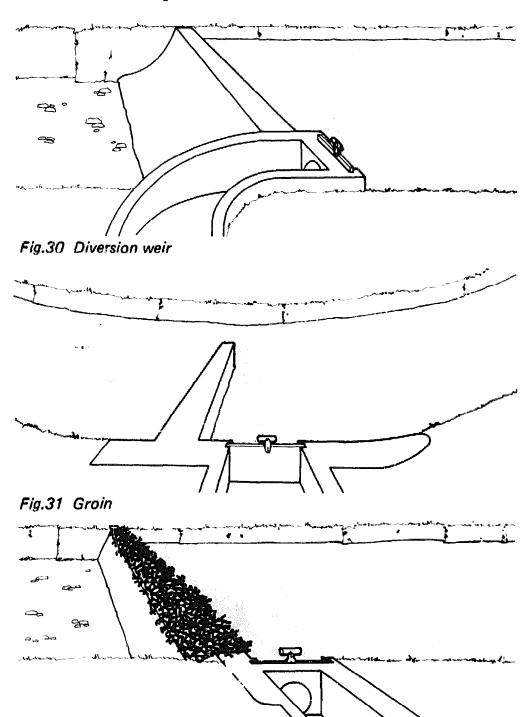
Fig.32 Low dam with washout section .
