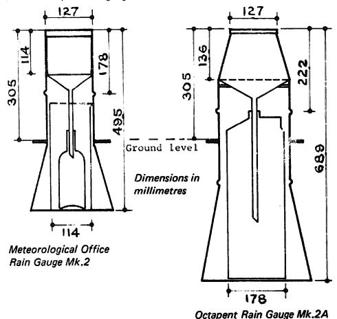
Fig. B2 Two types of British rain gauges
