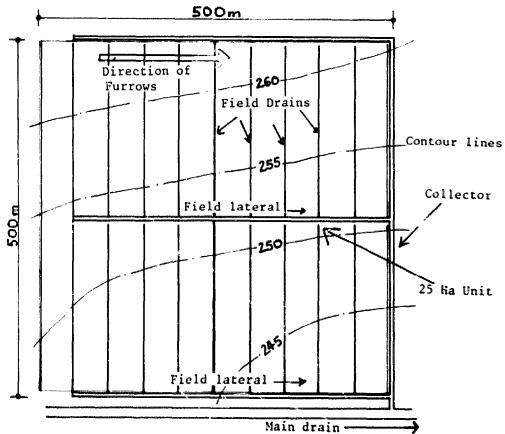
Fig.26 Drainage layout for a 25-hectare farm unit
