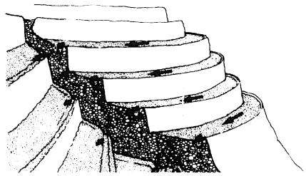
Fig.11 Drainage of terraces
