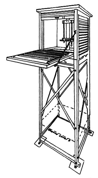
Fig. B3 Ordinary thermometer screen on steel stand
