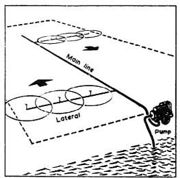
Fig.21 Simple sprinkler layout (Illustration: Wright Rain)
