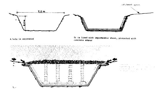
Fig.29 Catchment tank construction
