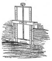
FIG. 45-THE STOKES MEASURING GATE.
