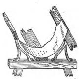
FIG. 36—END VIEW OF SMALL IRON FLUME.
