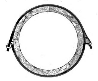
FIG. 27-CROSS-SECTION OF STAVE PIPE.
