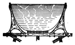
FIG. 37-CROSS-SECTION OF LARGE IRON FLUME.
