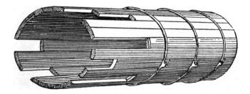
FIG. 26-SIDE VIEW OF STAVE PIPE.
