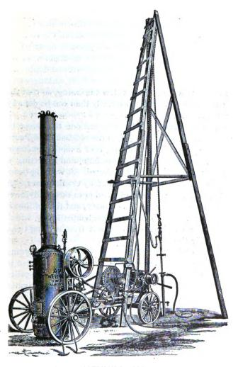
FIG. 94-ARTESIAN DRILLING OUTFIT.
