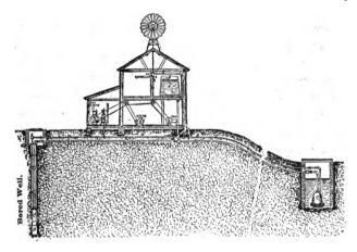
FIG. QI-THE PNEUMATIC SYSTEM.
