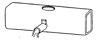
FIG. 54-SECTION OF VITRIFIED HEAD DITCH.
