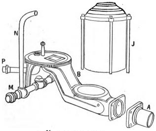
FIG. 86-HYDRAULIC RAM IN PARTS.
