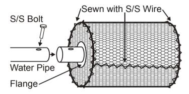
At the inlet of the pipe, a filter should be installed. A screened box can be used with the pipe entering one side, or add a considerable section of pipe drilled full of holes wrapped with screen or small holes and used without screen. The larger the surface area of the filter, the less flow restriction that will cause and the less likely the filter will be totally clogged with debris that has been sucked onto it. Make sure that the filter holes are smaller than the smallest nozzle used.
