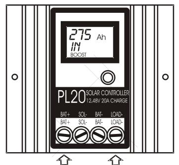
Resistive Load is connected between these two terminals (Or relay turned on/off by these two terminals)
