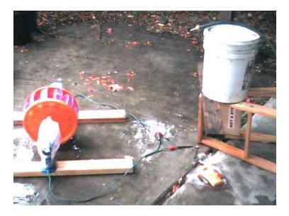
Next I tested output for two sets or 24 cups making two water wheels driving two 14.4 volt cordless drills. I measured between .5 to 2.9 amps (or .8 to 5.2 watts) charging one cell. Both generators were wired in series.
