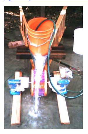
I also tested a 1/8" water hose nozzle blasting water out at city water pressure (about 45 lbs/Sq. Inch). This approach would charge two cells at about .45 amps and one cell at about .5 amp or .8 watt. This approach uses the inertia of the water. Both generators were wired in series. See <u>http://home1.gte.net/mikelob/WaterW-9.JPG</u> for the setup.
