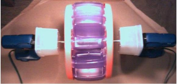
Stack one plastic container on top and nested in the lower one. Drill in a hole in the middle of one of the longer sides. Use a #8-32 by .5" long machine screw and nut to fasten them together. The containers are positioned so the overlap is just barely enough to bolt them together. See <a href="http://home1.gte.net/mikelob/WaterW-1.JPG">http://home1.gte.net/mikelob/WaterW-1.JPG</a>
