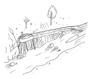
Simpler than a dam, it is most suitable for small villages or isolated houses. It also avoids the worst of flooding as most of the stream flow will follow the main stream channel.
