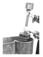
side. You will notice from the sound and gentle vibrations that PowerPal begins working immediately. If you do not notice this then there is a problem with your site. Check again that you have followed the initial procedures correctly. The lower bearing is lubricated by water so water must be allowed to enter the lower hole drilled in the shaft tube.
