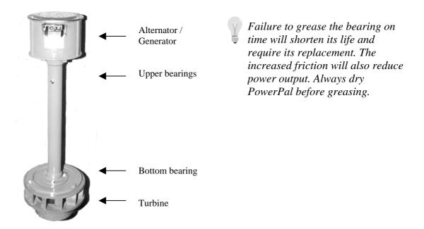
\* Note – this applies to models MHG-200LH & MHG-500LH. If you have purchased model MHG1000-LH you may find one of the upper bearings located above the generator and one below the generator. The bearing below the generator requires greasing (near the grease nipple).
