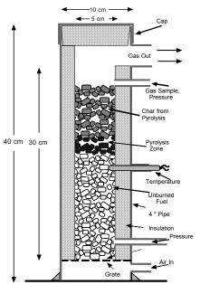
Figure 1 – Gasifier for measuring effects of superficial velocity change.
