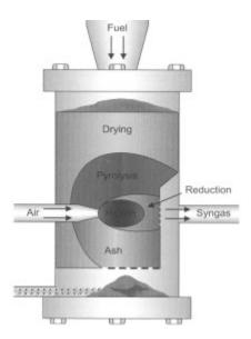
In a cross draft gasifier the air enters from one side of gasifier reactor and gas is taken out from other side. The cross draft gasifier is one of the simplest gasifier designs. It has a quick start time and reaches high temperatures which may require air or water cooled nozzles.
