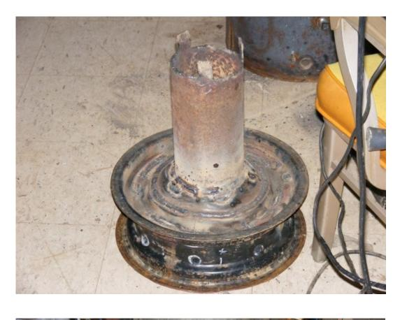
Rim completed. All holes welded closed. Pipe is 5" diameter 11.5" long. Rim is 14"
