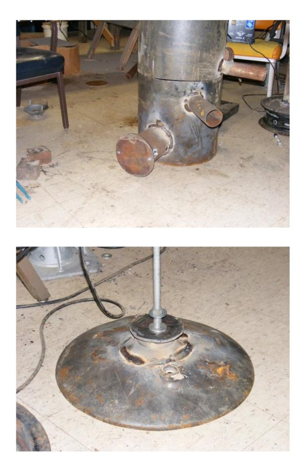
Ready to weld all thread to hold tank together..
