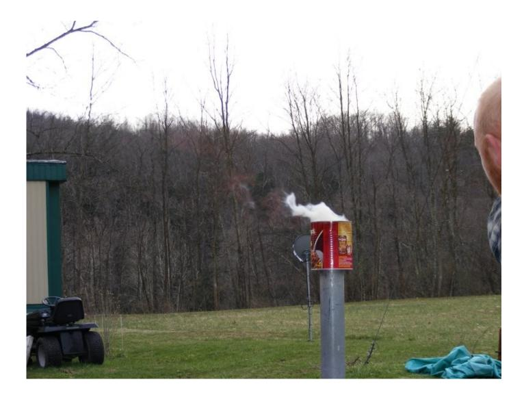
The first flame from the gasifier as this was the first test ever did on this unit after we built it. You can see some orange in the flame looking through to the trees in the back ground. This flame is about 3 to 3-1/2 feet coming from a 3" pipe. A 1 gallon can is used to stop cross winds. This flame is very hot at this point.
