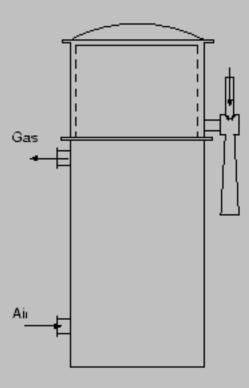
Figure 2: Drying of fuel with an ejector.
