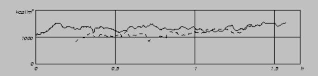
Figure 8: Test with cooled and uncooled monorator container, using wood of about 45 % moisture.
