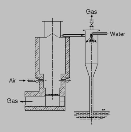
Figure 1: Gasifier at Outokumpu copper mill.
