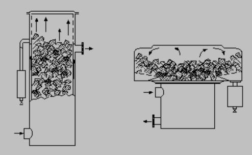
Figure 5: Gasifier, to the left a standard model, to the right with monorator container.
