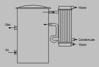
Figure 3: Drying device suggested by Lutz.
