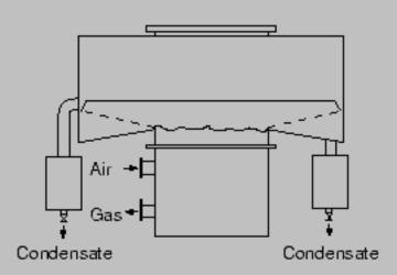
Figure 9: Test-device for examining cooling effect.
