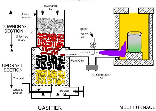
THE UP-DOWNDRAFT GASIFIER FOR METAL MELTING "THE DASIFIER"
