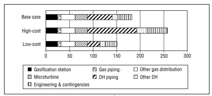
Figure 4. Total initial cost by component for the village trigeneration system (10<sup>3</sup> 1998 \$)
