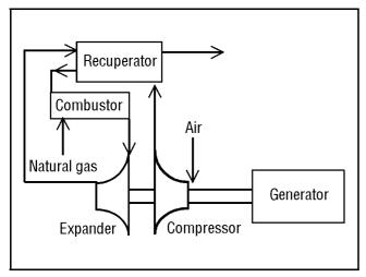
Figure 1. Recuperated microturbine fueled with natural gas
