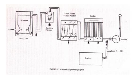
There is quite a substantial pressure drop across the whole gasification system and the design is usually done such that the pressure drop should not exceed 100 cm of water<sup>7</sup>.
