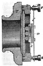
Fig. 51.—Scale 1. Granulated Carbon Transmitters.—These are undoubtedly the most powerful for
