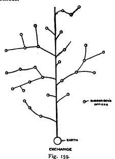
The difference is shown by Figs. 158 and 159, the former of which represents the Law and the latter the Mann call wire for joining up the same 31 stations.
