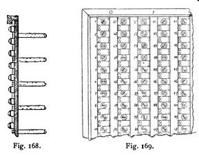
panel for 600 lines. The numbering is from top to bottom of the panel. The projecting pins at the back, covered with vulcanite sleeves, are used simply to form troughs to guide the wires and keep them tidy.
