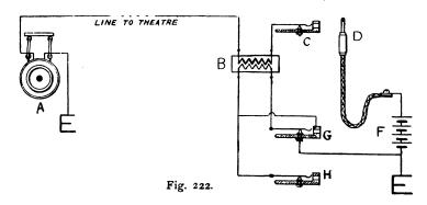
connected by a plug and cord, or a metallic circuit line may be connected and the earth cut off by plugging a double plug and cord into G.
