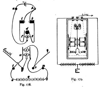
which also shows the connections. A double battery is required for this, as shown.
