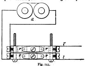
screws shown. Two holes are drilled in each plate, those in the front one large enough for the outside of the plug, and those in the back one for the small part of the plug. The connections to the drop a and to the lines l l' are shown in Fig. 155. The springs r r are furnished with phosphor-bronze pins, which project slightly into the plug holes, and ensure good contact on to the plugs when these are inserted. No contacts are broken when the plug is inserted, a derived circuit
