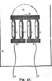
the less sensitive will be the instrument, owing to the increased pressure at the carbon contacts.
