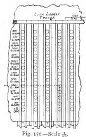
right angles. Connections between the two are made in a special manner, designed to keep the wires used for the purpose in an orderly condition, and that they can readily taken out and others run between different points of the boards. This is managed in the following manner:-In a vertical line over each of the troughs TT, Fig. 163, a series of fourteen 4-inch holes are bored in the framework, as shown in Fig. 170. The connecting wires are
