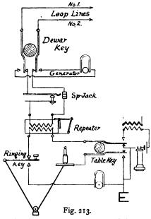
Coleman-Jackson translator. It will be seen that the local circuit of the translator is not complete when the line is not in use. This arrangement is adopted because the drop is much more sensitive under such circumstances. A test cell for multiple testing is shown also in Fig. 213.
