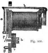
a lever attached at right angles to the armature, which is placed very near the cores of the magnet e. These cores at the other end are attached by iron screws to the strip of iron, d d (shown in section), which forms the yoke and support for some five or ten drop indicators. Along the back of d d a strip of ebonite, i, is attached, and through this and underneath the centre of each drop a screw, h, projects to the front through a hole drilled in d d.
