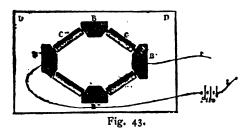
be seen that the current divides into two branches having two pencils in each. The instrument is not so powerful as others of the class, owing probably to the high resistance of the primary circuit.
