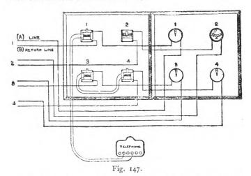
Fig. 147 shows the connection for four lines, the indicators at the right and the connecting jacks at the left. Lines 3 and 4 are shown connected together with both indicators left in circuit. Line I is shown connected to the operator's set, and line 2 normal.
