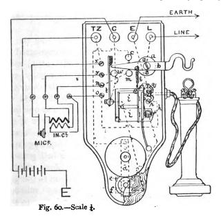
d, stud c, lever b and a to line, and through the signalling apparatus at the other end and back by way of earth to the battery.
