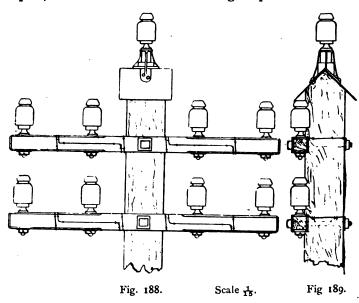
The arms, which are usually of good sound oak, about  $2\frac{1}{2}$  in. square in section, are fitted into grooves sawn on one side of the poles at about 12 inches apart, and are secured by a bolt which passes through pole and arm, as shown in Figs. 188 and 189, which also show the *pole roof* of galvanised iron fitted on the top of a pole and surmounted by a *saddle bracket*, into which the bolt
