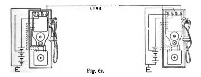
Fig. 62 shows two instruments connected up to a line, and forming a complete private installation.
