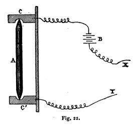
C C' are attached to a sounding-board of thin deal, wires being connected to C C' for joining up the battery and receiver. The complete instrument is shown in Fig. 23, and forms the parent of a very numerous class of telephone transmitters; indeed, nearly all transmitters in use are but modifications or amplifications of some form or other of Hughes's microphone.
