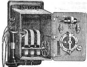
Fig. 85 shows a useful form of movable desk magneto set, made by the Consolidated Telephone Company.
