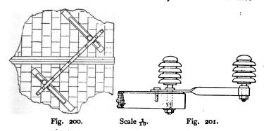
four wire arms, and four wire arms into six, the extending piece being of wrought-iron formed into a boss at one end.
