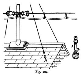
tances of every 3 or 4 feet by suspenders, which are either made up of short lengths of stiff wire, or, what is better, and has come much into use lately, by short pieces of raw hide attached to a hook or ring, which is threaded on the suspending wire, as shown in Fig. 204, which also shows the cowhide, etc., on a larger scale at A.
