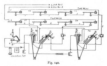
free, she inserts the plug, and to ring him up depresses the button a, so as to bring the spring  $d^3$  on to battery or generator contact  $d^5$ . After thus connecting, the operator cuts out her own instrument by pressing the ebonite block d under spring  $d^1$  by means of the button a.
