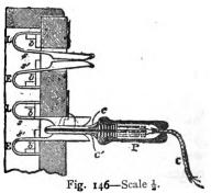
ment into a kind of flat spring-jack, both being shown in Fig. 146. CC' are two strips of brass fastened on
