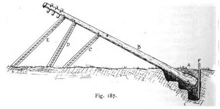
out about eighteen inches wide and four or five feet long, the longest side, if possible, being parallel with the line of the wires to be erected. This space is then dug out in steps until the end where the pole is to rest has reached the proper depth.
