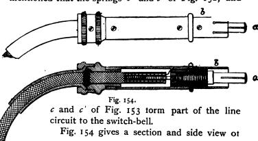
the double plug used at the central office to make the connections.
