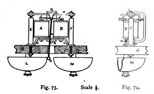
Action.—The effect of passing a current through the coils is to strengthen the north polarity of one core, and to weaken or altogether neutralise the north polarity of the other core, the effect being that the armature is strongly attracted to one core and not at all by the other. The next reversal of current causes the core which was strengthened before to be weakened, and vice versa, so that the armature vibrates over to the opposite
