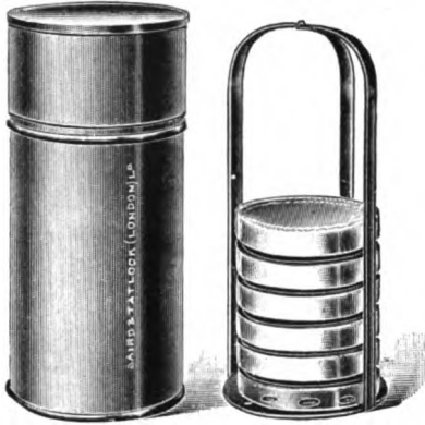
FIG. 1.—Copper cylinder with deep overlap in which to sterilize Petri dishes.
