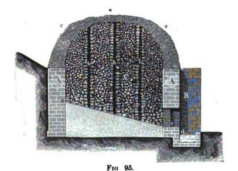
sulphur is gradually melted, and running away by the opening (a) at the bottom of the heap, is cast into moulds. By this process, which takes several weeks to complete, the richest ores, containing from 30 to 40 per cent., may be made to yield from 20 to 25 per cent. of sulphur, whilst common ores, containing from 20 to 25 per cent., yield from 10 to 15 per cent. of sulphur, the remaining portion of the sulphur being used up for combustion.
