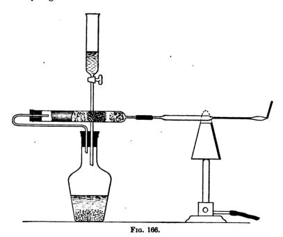
dilute hydrochloric or sulphuric acid, great care being taken to have these materials free from arsenic. Before adding the arsenical solution the hydrogen is evolved for twenty minutes, the shoulder of the reduction tube being meanwhile heated to redness, as shown in the figure; if no mirror of arsenic be formed in the fine portion of the tube in this time, the materials may be assumed to be free from arsenic.
