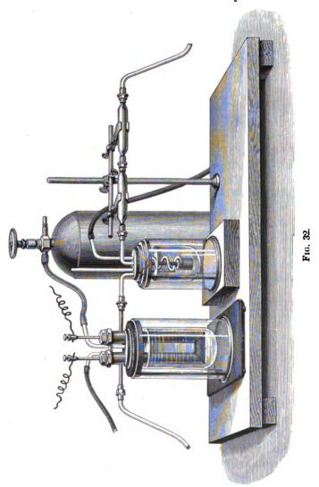
but the platinum electrode at which the fluorine is liberated is much corroded with formation of a certain quantity of a black powder consisting of platinum fluoride. The volume of fluorine obtained with this apparatus is from three to four litres per hour. Copper vessels may also be employed in place of platinum, but the electrodes must consist of the latter metal.<sup>1</sup>
