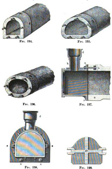
end elevation in Fig. 198, is attached to the open end or ends of the retort by means of bolts, and when the charge has been added, the end of the mouthpiece is closed by an iron lid,
