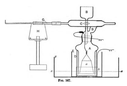
in the Government laboratory, depends upon the fact that when hydrogen is evolved electrolytically in the presence of arsenious acid or its salts arsine is formed. Arsenates are not reduced in this way and must be reduced to arsenites before being treated by this method.
