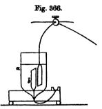
683. Electrotype.—There are several modes by which metals may be deposited by means of electricity on
