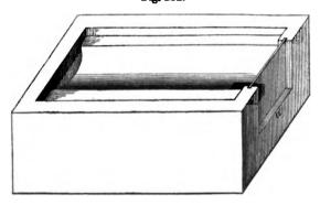
which is exceedingly well adapted for eudiometrical experiments. It is made of wood, and has a piece of plate-glass inserted at a, by slipping between two grooves. It does not require so much mercury as would appear from its size.
