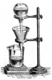
fig. 113, in such a manner that the neck of the flask is below the water; in this position no water escapes from the flask until the liquid in the funnel falls below the neck; when this takes place, a bubble of air enters and an equivalent bulk of water escapes, and the washing proceeds slowly in this manner, until the whole of the liquid has passed through the precipitate.
