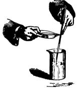
to slowly raise the vessel until the fluid meets the glass rod; it will then run down it with perfect regularity, and may be directed even into the neck of a small flask as conveniently as by the use of a funnel.
