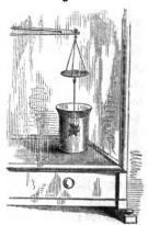
and if we now place weights into the short pan until the equilibrium is restored, they will express the weight of a volume of water equal to that of the substance. For example:—
