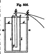
by keeping crystals of the latter salt upon the perforated shelf, dd. The zinc rod must be amalgamated. When this battery is first charged, it is more powerful than it is afterwards, but after the first quarter of an hour it will remain quite uniform for several hours.
