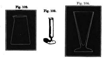
a considerable size. They are sometimes made of the same shape as that represented in fig. 103, but blown at the lamp and exceedingly thin, and thus resemble a test-tube on a foot; they are very convenient in many experiments of a delicate character.
