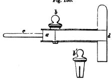
is held by one of Gahn's cylinder-holders, an excellent contrivance, the structure of which is seen by reference to fig. 138.
