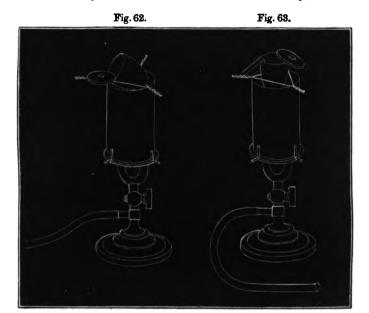
more combustible gases are evolved, when the crucible may be arranged in the position seen in figs. 62 or 63, preferably the latter.
