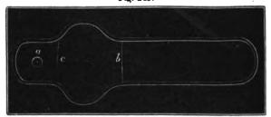
be passed into the gas-jar. There are also two recesses, to enable the thumb and finger to enter the trough, to manage the tube used to introduce the reagents alluded to. 519. It is essential to use these troughs upon a tray, in order
