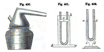
fixed at their lower extremities into a foot. On their upper ends they carry small semicircular brass pieces, ab, which hold the U-tube. The wires are somewhat nearer together than the width of the tube, so that a little force is required to insert it in its place, thus giving greater firmness to the apparatus.
