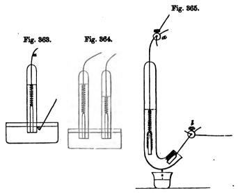
in the fluid, the oxygen will be obtained in the tube. If the hydrogen is required, it will be necessary to reverse this arrangement. Fig. 364 shows another mode of obtaining both gases in separate tubes.
