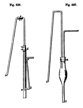
being, that as the caoutchouc junction allows a certain amount of motion, the chances of fracture are much diminished; and, moreover, if the instrument be broken at the bend which unites the longer and shorter leg, another tube has merely to be bent and inserted into the tube, d a. In many cases the two limbs
