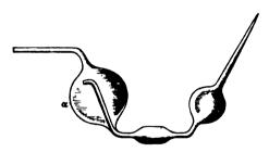
is plain that if regurgitation should take place, the acid merely enters the bulb, a, without finding its way into the combustiontube. The acid for condensation is chiefly contained in the smaller bulb, a little being, however, allowed to enter the other. On the 5th of the same month, Mr. Warren De la Rue described a similar instrument which he had been in the habit of using for eighteen months previously; the same idea appears, therefore, to have
