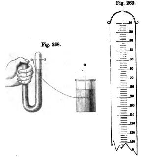
the jar. On bringing the other wire of the eudiometer in communication with the interior coating of the jar, by means of the knob of the latter the spark passes and inflames the mixture.
