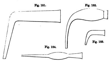
If it is merely desired to connect the exit of a Liebig's condenser with a bottle or flask intended to contain the distillate, figs. 181, 182, and 183 are the best; but, if the fluids being distilled do not require much refrigeration, and it is simply intended to connect the retort or other distilling apparatus with the receiver, figs. 184, 185, and 186 are convenient. It is
