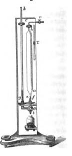
The first of these indicates the method of opening a communication between the pipette, b a, and the tube, g h. In the second, the tube, g h, and the pipette communicate; and, at the same time, t being open, the mercury is allowed to escape, for the pur-
