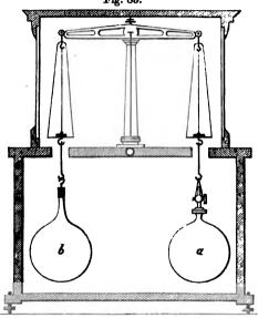
cemented to it a brass mounting, terminating in a hook, to enable it to be suspended from the balance-pan. If the united weight of the water displaced by the balloon, b, and its mounting is less by n grammes than the weight of the water displaced by the balloon, a, we must attach to b a glass tube closed at each end, and having an exterior bulk = n cent. cub. of water.
