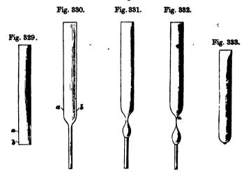
The tube is to be strongly heated at one end, from a to b, fig. 329. Another piece being then attached, the heat is to be directed at a b, fig. 330, the tube being continually rotated, in order to equalize the heat; it is then drawn out, as at fig. 331, and the flame being strongly directed at a, fig. 332, the superfluous glass is to be drawn off. The tube, after a little turning in the flame, then appears like fig. 333. The mouth is then
