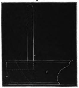
capable of admitting a glass tube 2 inches long by  $\frac{1}{2}$  an inch wide, to enable caustic potash or any other substance required to
