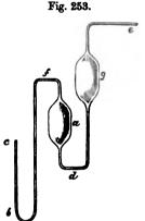
the same time the gas passes through cb and f into a. As it is now essential that the tube, bc, should be closed, that is done, if the gas alluded to stands over mercury, by merely depressing the aperture, c, beneath the surface of the metal, and applying a slight suction to c.
