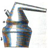
hand, to cohobate in the manner shown in fig. 208, I have the copper cover, fig. 399, attached to the pot. It is to be luted in the same manner as the head, fig. 398.
