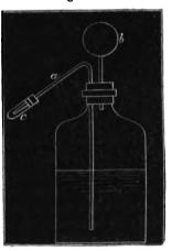
On applying pressure to the ball, the solution rushes up the tube a, and is forced into the burette or other vessel used to receive it. On removing the hand, the ball resumes its original shape, and a volume of air equal to the fluid expelled enters by a. The fact
