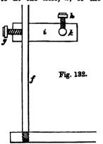
The instrument is particularly applicable to the support of small retorts during distillations, and in fact is constantly useful where vessels have to be supported at varying heights.
