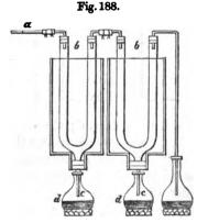
and terminate in the flasks, dd, which may likewise be placed in a freezing mixture.
