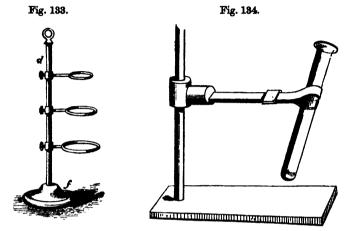
Distillatory apparatus, constructed of test-tubes, may very conveniently be supported by means of the tin test-tube holder, fig. 134. There it is seen that steadiness is obtained by means of the friction of a perforated cork enclosed in a tin cylinder, and sliding upon the rod; while the support for the tube is made to grip by slipping the piece of tin along the clasp. This is a cheap and useful piece of apparatus, and may be constructed with ease out of pieces of tin and a few corks.
