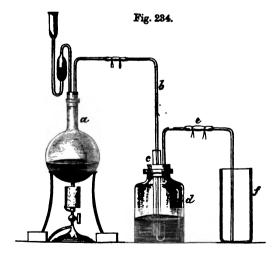
where a represents a flask in which the gas is prepared, which
