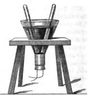
not to be used in eudiometrical researches, the boiling of the water may be omitted, and ordinary acidulated water be used instead. Of course the current must be allowed to pass until all the air is expelled, before collecting the gas.
