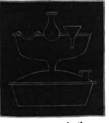
gin (fig. 53), contrived by Dr. Ure, may be conveniently employed. Its construction is obvious: the apertures are intended to hold flasks, capsules, or other vessels to be exposed to the heat.
