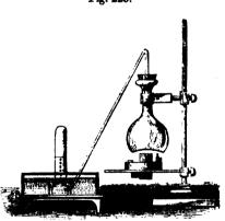
with the use of the cumbrous pneumatic trough, any basin or water-tight box answering the purpose. The water should be poured in until it covers the shelf for about an inch, when the jar, full of water and inverted, may be placed upon it, and supported, if necessary, by a ring of the retort-stand, or by Gahn's cylinder-holder, described at p. 161.
