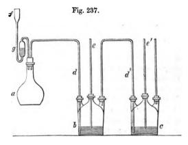
fitted a perforated cork; a tube passes from this into a little water contained in the first bottle, b, intended to wash the gas and retain any impurities mechanically carried over; from this another tube proceeds into c, which contains the water to be saturated, and thence, if necessary, into one or two more bottles. The
