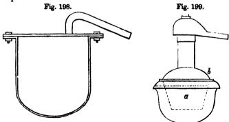
377. Where destructive distillation is to be performed on a much smaller scale, as in preparing aniline from indigo, chinoline from cinchonine or quinine, trimethylamine from narco-
