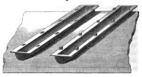
over it as soon as it acquires sufficient consistence to permit of being inverted without the paste falling out. The two are then wedged together, as in fig. 313. The mould is perforated in many places
