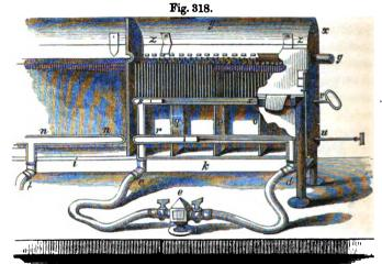
h and i are simply rectangular iron boxes, open at the bottom and covered at the top with wire-gauze, which are supplied by a horizontal perforated gas-pipe,
