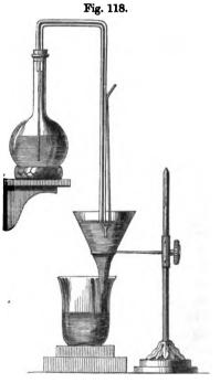
sufficiently high fo close the opening of the wider tube, the air no longer is able to enter the flask and the flow ceases. As the water passing through the precipitate falls in the funnel below the opening of the wide tube, the flow again proceeds, and so on, until the whole of the water in the flask has been expended.
