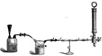
render it tight. A slight vacuum is produced by making a stroke of the piston, and the tap, s, is to be turned off. A strong blowpipe-flame is now made to play upon the parts d and b which are to be closed, the operation being greatly facilitated by the vacuum.
