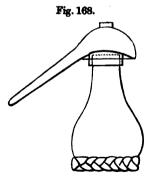
was a gourd-shaped vessel (whence one of its names, cucurbit), well fitted for being cleansed, or to have solids or liquids introduced. The head, or capital, was also singularly perfect in shape for the intended uses; it had a species of channel all round to carry any liquid which condensed in it to the beak, by which it was conveyed to the receiver. Modifications of the alembic are still used, and will be pointed out in the proper place.
