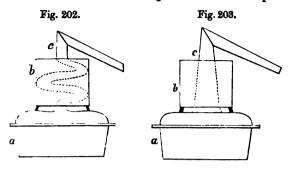
the receiver. Sometimes it is unnecessary to have a worm passing through the water, a rather considerable elongation of the head being sufficient to prevent the passage of fluids of high boiling-points, as in fig. 203.
