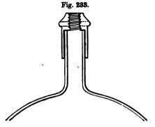
med paper. If at the end of an hour or so the water has not fallen, the cap and its adjuncts are perfect.
