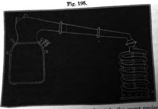
worm should be inserted into a wooden tub, the spout projecting at the bottom. This is the most easily fractured part of the apparatus, and requires especial care. It is a good plan, as a means of protection, to have two stout results of wood nailed to the tub, and standing out to the
