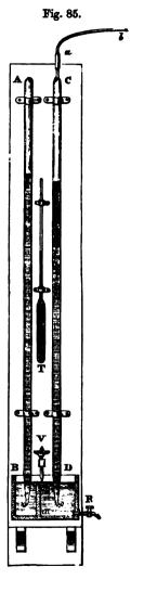
into two parts, the smaller of which serves for the cistern of the barometer. Into the second compartment is plunged the tube, CD, which has the same diameter as AB. CD is capable, by means of a leaden tube, ab, of being placed in communication with the balloon.
