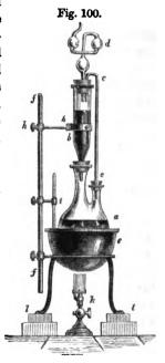
vegetable matter, it falls back into the flask, to be again raised as before. The three-bulbed apparatus, d, acts as a safety-tube, and also serves to condense any of the spirituous vapour which might otherwise be lost. The digesting vessel, b, is supported by the clamp, h h, which slides on the rod, ff. The gas-burner, k, enables the temperature of the bath to be regu-
