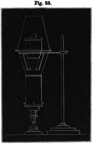
and others, that it is seldom necessary to use Sefström's blast-furnace. Where the full powers of a lamp are required to be exerted, the crucible jacket, fig. 33, is necessary; it will be seen that the crucible is supported on three knife-edges; the arrangement is such that the flame is made to act on the crucible in a manner well adapted to economize the heat and avoid loss by radiation.
