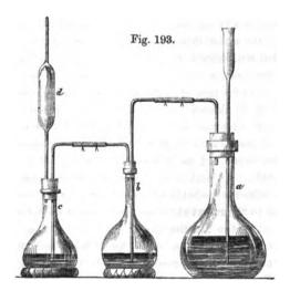
363. It has already been mentioned, at p. 225, that fluids distil at a lower temperature in a current of hydrogen than when
