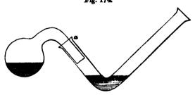
very useful. The fluid to be distilled is made to occupy the part a, and gentle heat is applied just sufficient to raise the vapour,
