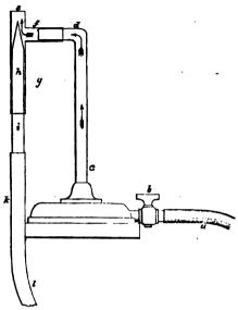
supply by means of the flexible tube, a, it may be readily adjusted upon the laboratory table.
