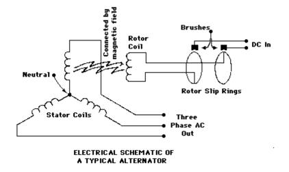
A modern alternator contains both moving and stationary coils of wire. In the alternator, however, the moving coil, called the rotor, uses current supplied through slip rings to generate a moving field. Power is extracted from the stationary field coils.
