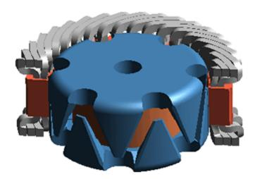
In the picture above, of the two blue claw-pole rotor pole pieces (with the shaft removed) can be seen nested in their normal operating position within a cutaway view of the power producing three phase stator coils. Note the orange donut shaped powerful permanent magnet that now replaces the old electromagnet coil sandwiched between the two claw shaped rotor pole pieces.
