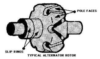
THE (SIX POLE) CLAW POLE ROTOR DESIGN PRODUCES 12 ALTERNATIONS IN THE MAGNETIC FIELD PER ROTATION PER SHAFT ROTATION, ALLOWING MUCH SLOWER SHAFT SPEED TO SUFFICIENTLY PRODUCE THE REQUIRED MAGNETIC FIELD "ALTERNATIONS"
